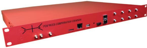
The Per Vices Crimson SDR has 4 independent receive chains and 4 independent transmit chains, each capable of as much as 322 MHz of RF bandwidth up to 6 GHz.
