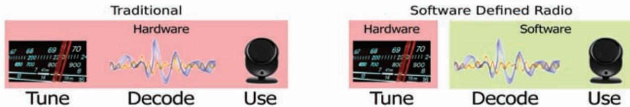
● ● Figure 2: Comparison between the traditional approach for wireless devices, where all functionality is done in hardware, compared to SDR where only the tuning is done in hardware and the decode and use is done in software giving a much more flexible system.
